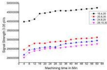
Fig. 7. Measured Signal strength for different machining time at a constant current 3 amps for Stavax material
