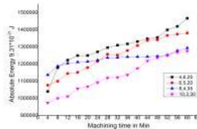
Fig. 5. Measured Absolute energy for different machining time at maximum Pulse on of 28 $\mu$ s for stavax material
