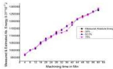
Fig. 17. GMDH estimates of Absolute energy for various percentages of data in training set for stavax material
