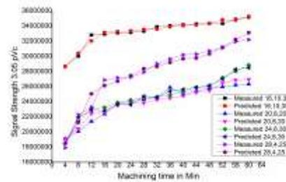
Fig. 13. Regression analysis estimates of signal strength for various machining time for maximum current 6 amps for stavax material
