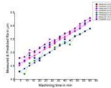
Fig. 8. Regression analysis estimates of surface roughness for various machining time for Maximum pulse on 28 μs for Titanium material
