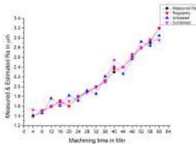
Fig. 15. GMDH estimates of Surface roughness for 50% of data in training set for stavax material
