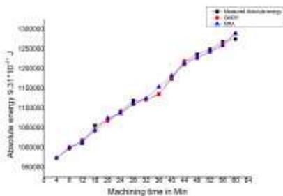
Fig. 19. Comparison of GMDH and multiple regression estimates of absolute energy for Stavax material
