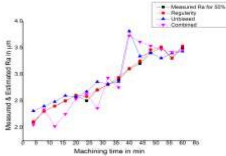
Fig. 14. GMDH estimates of surface roughness for 50% of data training set for titanium material
