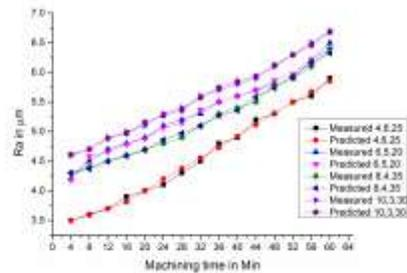
Fig. 9. Regression analysis estimates of surface roughness for various machining time for Maximum pulse on 28 μs for Stavax material
