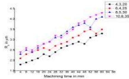
Fig. 2. Measured surface roughness for different machining time at minimum Pulse on of 16 $\mu$ s for titanium material
