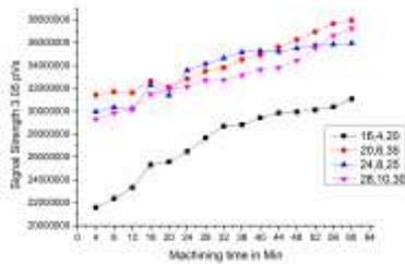
Fig. 6. Measured Signal strength for different machining time at a constant current 3 amps for Titanium material
