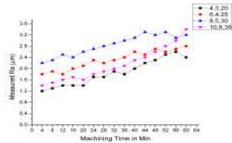
Fig.3. Measured surface roughness for different machining time at minimum Pulse on of 16 $\mu$ s for stavax material
