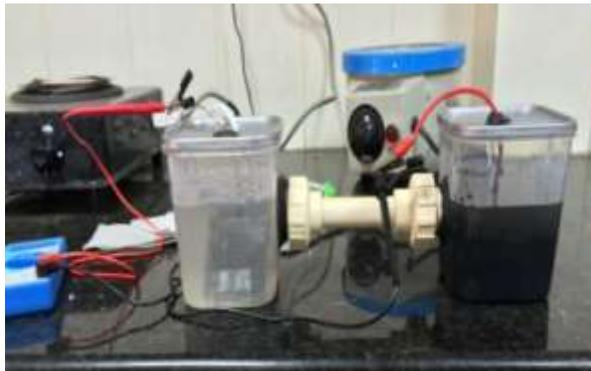
Figure 1: A prototype model of the MFC
