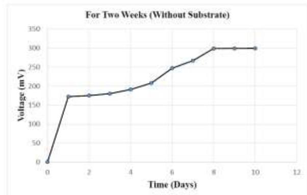
Figure 2: Voltage v/s Time of MFC without Substrate
