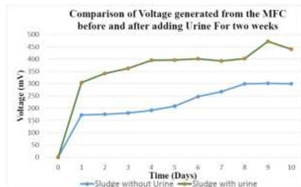
Figure 3: Voltage v/s Time of MFC without and with Urine
