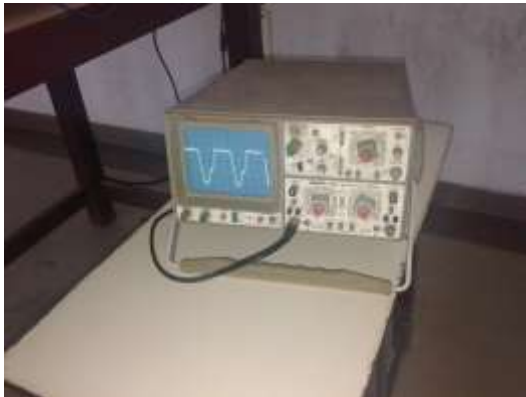
Fig. 13(c) Waveform of energized circuit with 30 V input
