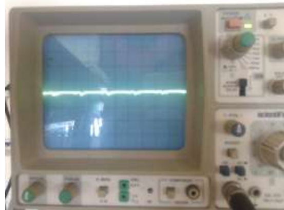
Fig. 12 Waveform of an un-energized circuit
