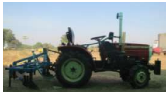
Plate 1: Modification in air intake system
