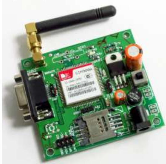
Figure 10 GSM Module SIM900
