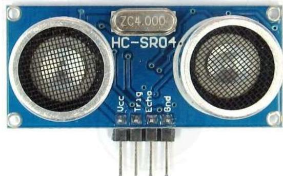
Figure 6 Ultrasonic Sensor HC-SR04
