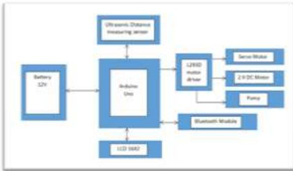
Figure 2 Robot Block Diagram
