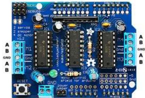
Figure 5 L293D Motor driver shield
