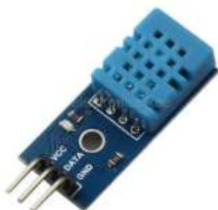
Figure 8 DHT11 Temperature and humidity sensor
