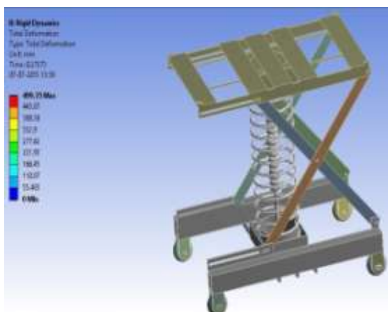
Fig 13 Total deformation of the assembly
