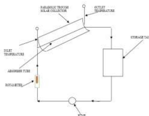
**Fig. 3.1** Flow Diagram of a Parabolic Trough Solar Collector
