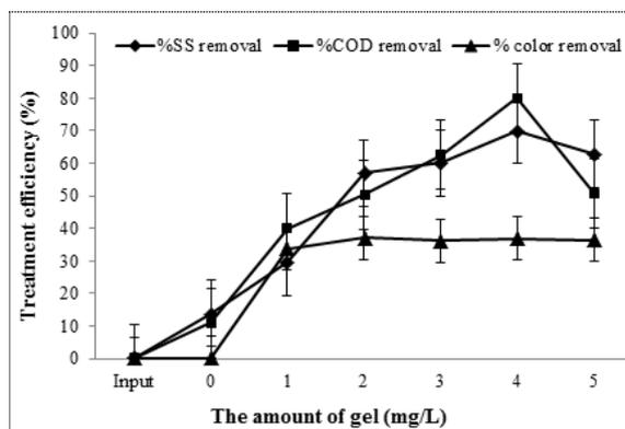
Figure 4. Treatment efficiency of the auxiliary coagulant gum MHY to the wastewater of factory 2
