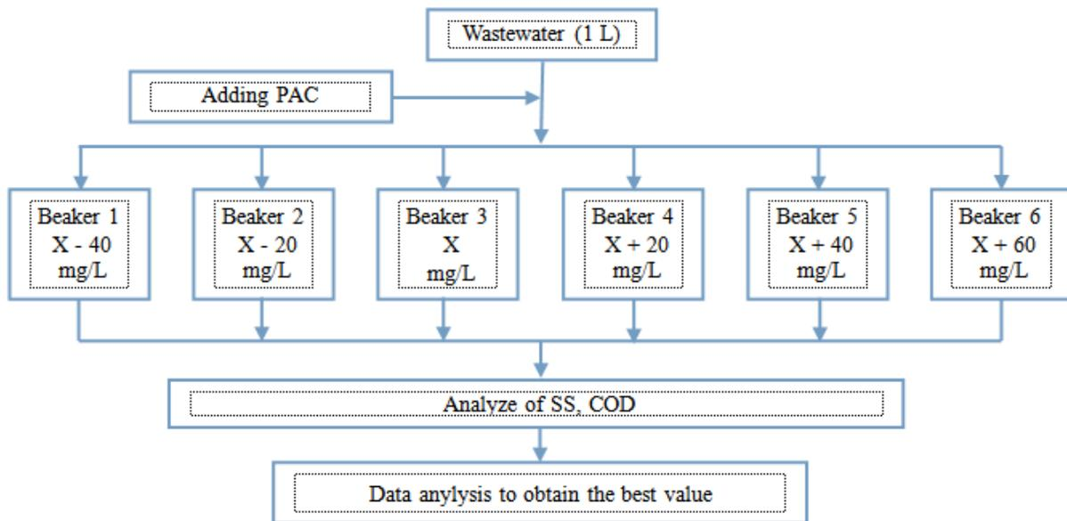
**Figure 1** Experimental arrangement to determine the amount of PAC (experiment 1)
