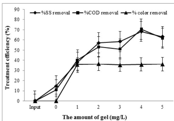
Figure 3. Treatment efficiency of the auxiliary coagulant gum MHY to the wastewater of factory 1
