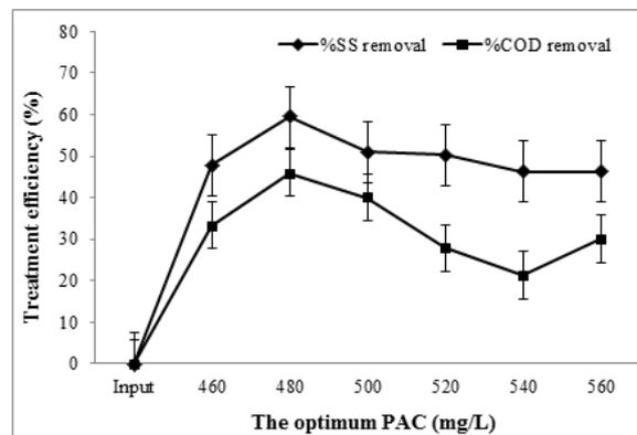
Figure 2. Efficiency in COD and SS removal at different concentration of PAC
