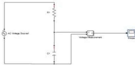
Fig.9 Circuit diagram for configuration 1 of integrator.
