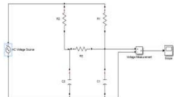
Fig.11 Circuit diagram for configuration 2 of integrator
