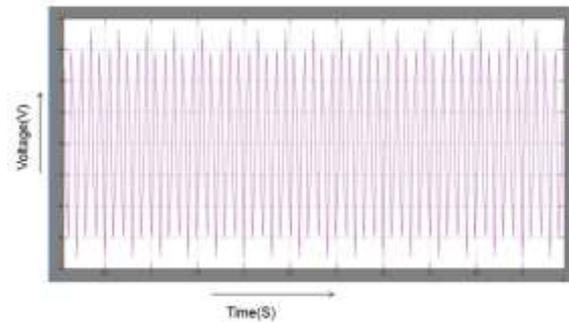
Fig.10 Output waveform for configuration 1 of integrator for 30V AC input
