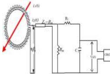
Fig..1 The Rogowski coil with a conventional RC.integrator.
