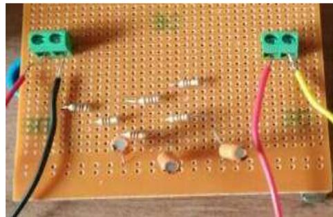
Fig. 18 Hardware circuit of efficient configuration of integrator circuit
