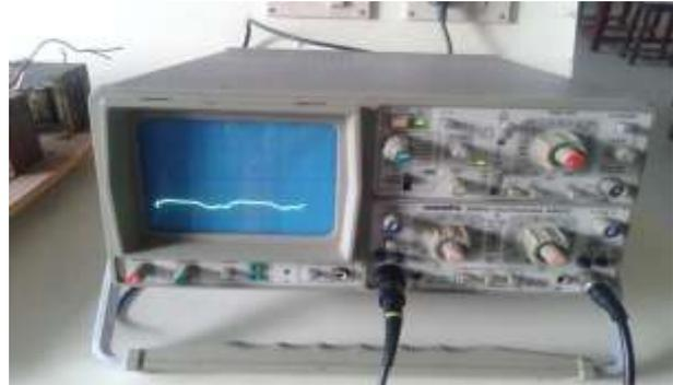
Fig. 22 Output of integrator
