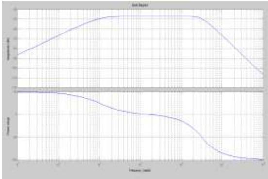
Fig.7 Bode plot for  $R=100\Omega, C=1\mu F$
