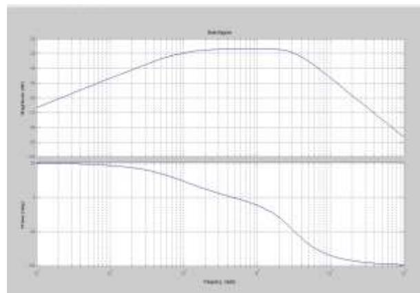
Fig.6 Bode plot for R=100 Ω, C=0.1μF
