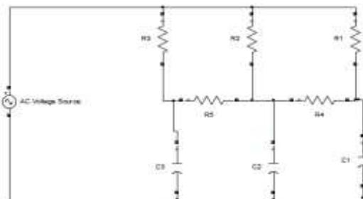
Fig. 5 Configuration 3 of Integrator circuit
