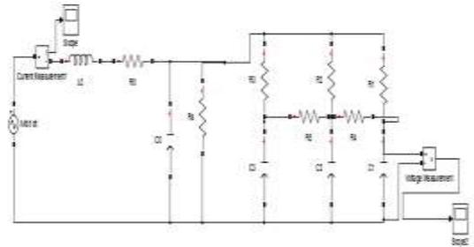
Fig.15 Lumped parameter model of Rogowski coil with a RC integrator
