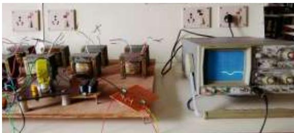
Fig. 20 Overall circuit of long duration impulse current measurement
