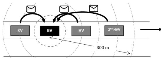
Figure 2. Proposed model of vehicle positions for message passing when maximum number of vehicles in a single line road segment. RV, BV, HV represents Rear Vehicle, Base Vehicle, and Head
