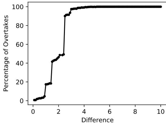
Figure 3. The dots represents the percentage of overtakes happened for each speed difference between two vehicles within 300m. According to the graph, it is possible to identify four levels of overtaking possibility. 0-1.5 low possibility of overtake, 1.6-2.5 average possibility, 2.6-5.0 high possibility of overtakes and 5.0 and above exact overtake.
