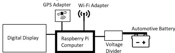
Figure 4. Block diagram of the prototype vehicle node.
