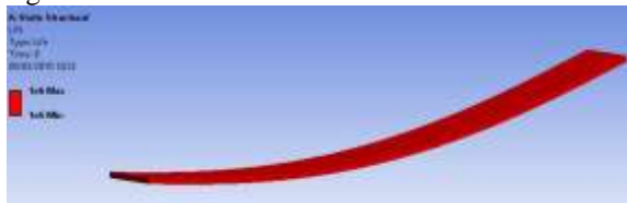
Fig. 4 Fatigue analysis of steel leaf spring under full load i.e. 5400N
