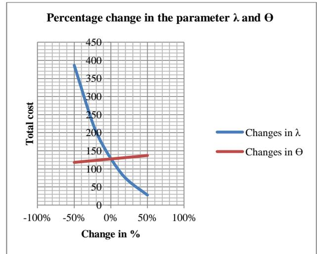
Figure 5 shows the sensitivity analysis in optimal total cost. It is observed that highly sensitive to changes in the parameter  $\lambda$  and slightly sensitive to changes in the parameter  $\theta$ .
