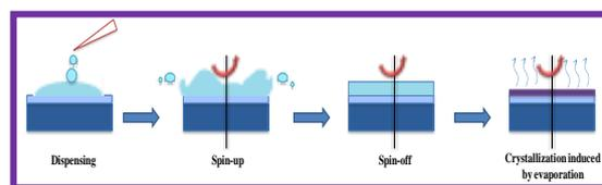
Fig. 2 Schematic illustration of typical stage of spin coating process
