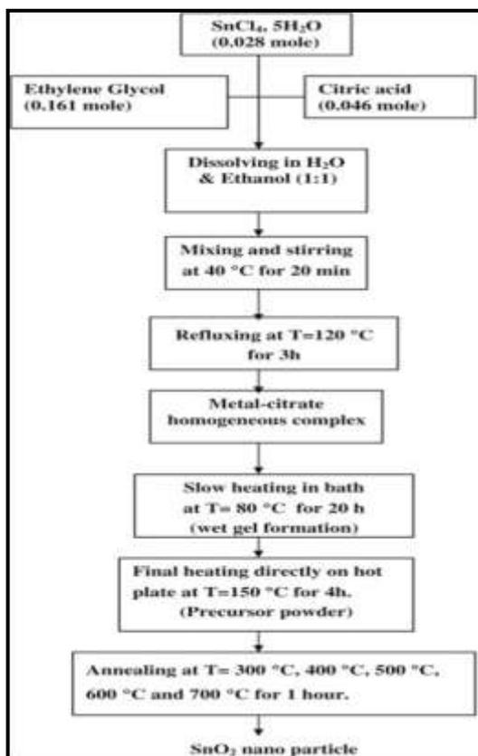
Fig. 1 Synthesis of SnO<sub>2</sub> particle
