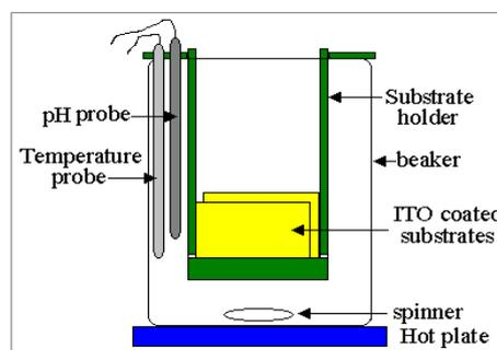
Fig. 3 Schematic illustration of Chemical bath deposition
