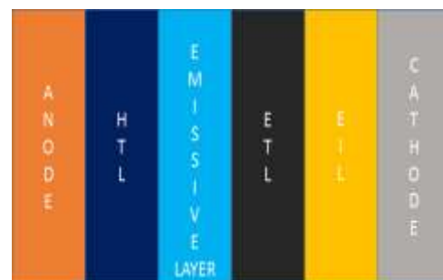
Fig.1 schematic device structure of OLED
