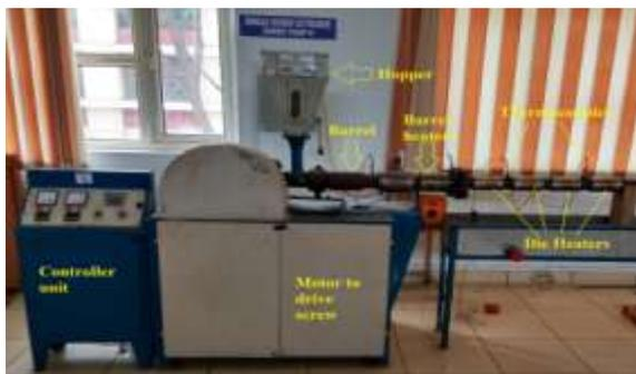
Figure 3: Single screw extruder
