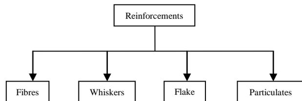
Figure 1: Common forms of reinforcements
