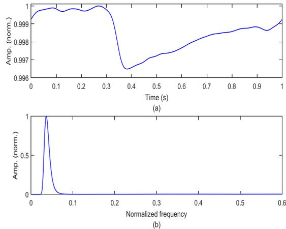
Fig. 11 Stockwell transform based plots during the event of feeder tripping in the presence of wind power generation (a) amplitude curve (b) normalized frequency curve.
