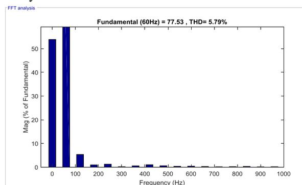
Fig. 15 Total harmonic distortions of current signal during the event of feeder reclosing in the presence of wind power generation.
