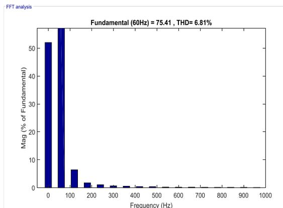
Fig. 12 Total harmonic distortions of current signal during the event of feeder tripping in the presence of wind power generation.
