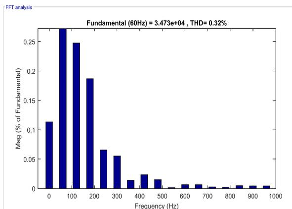
Fig. 13 Total harmonic distortions of voltage signal during the event of feeder tripping in the presence of wind power generation.
