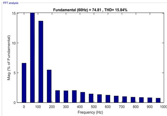
Fig. 6 Total harmonic distortions of current signal during the event of grid synchronization of wind generator.
