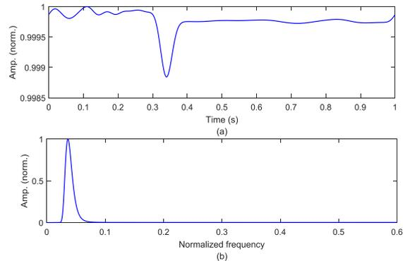
Fig. 8 Stockwell transform based plots during the event of grid outage of wind generator (a) amplitude curve (b) normalized frequency curve.
