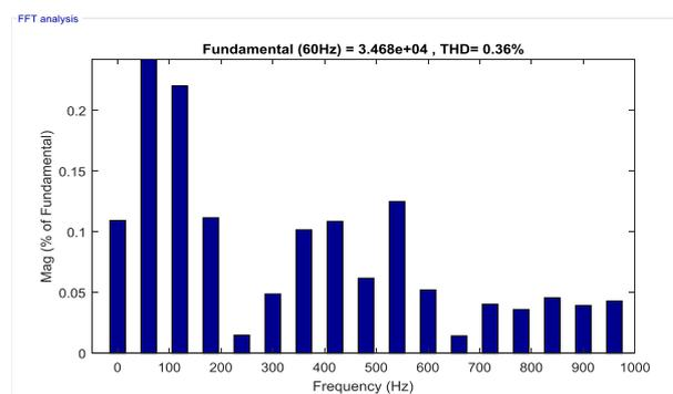
Fig. 16 Total harmonic distortions of voltage signal during the event of feeder reclosing in the presence of wind power generation.
