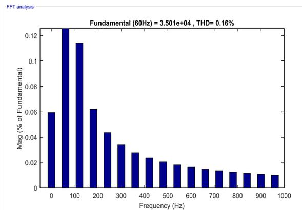
Fig. 4 Total harmonic distortions of voltage signal during healthy condition in the presence of wind power generation.
