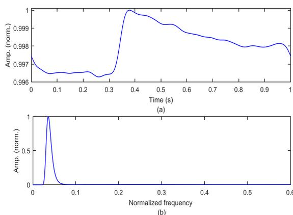
Fig. 14 Stockwell transform based plots during the event of feeder reclosing in the presence of wind power generation (a) amplitude curve (b) normalized frequency curve.
