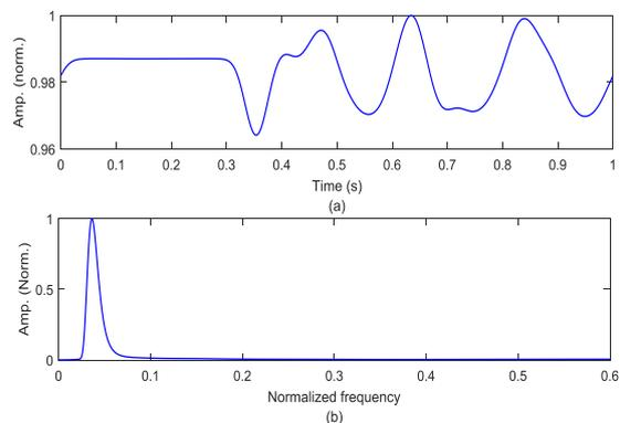
Fig. 5 Stockwell transform based plots during the event of grid synchronization of wind generator (a) amplitude curve (b) normalized frequency curve.
