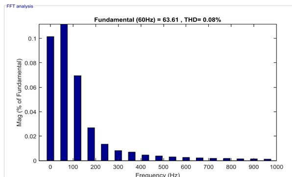
Fig. 3 Total harmonic distortions of current signal during healthy condition in the presence of wind power generation.
