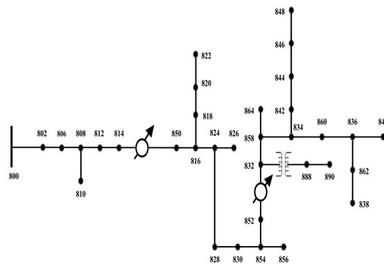
Fig. 1. Proposed IEEE-34 Bus Test System
