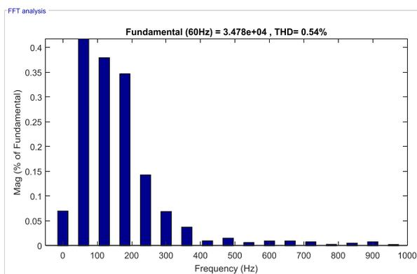
Fig. 7 Total harmonic distortions of voltage signal during the event of grid synchronization of wind generator
