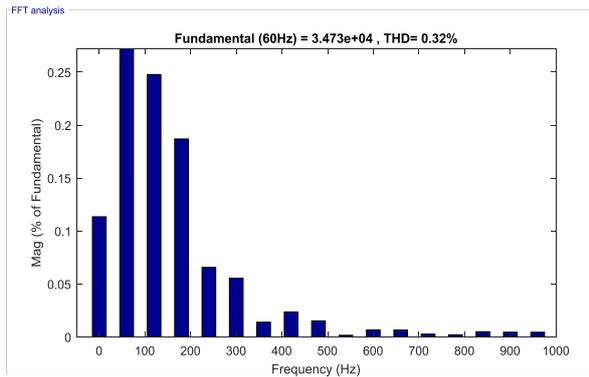
Fig. 10 Total harmonic distortions of voltage signal during the event of grid outage of wind generator.
