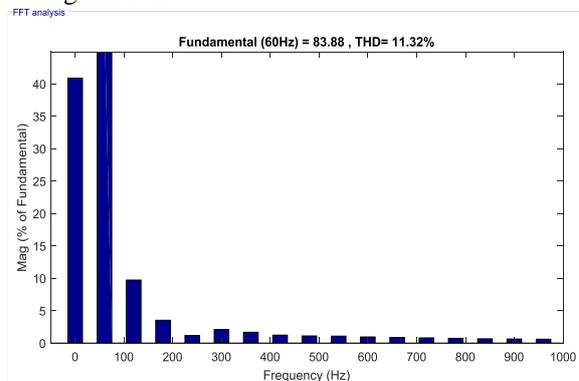
Fig. 9 Total harmonic distortions of current signal during the event of grid outage of wind generator.
