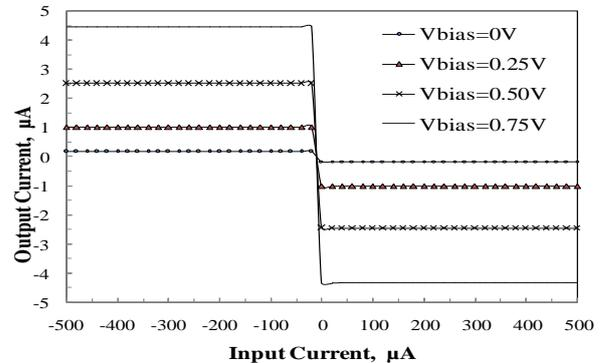
Figure-7 Current transfer characteristics of VCCCTA
