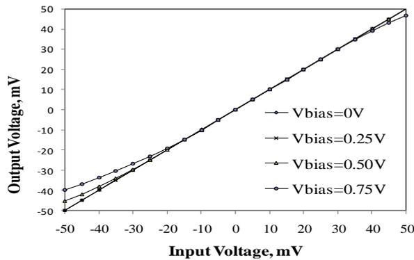
Figure-9 Voltage transfer characteristics of VCCCTA
