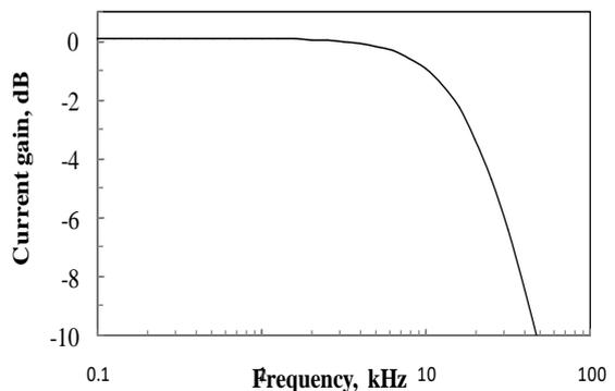
Figure-8 Frequency response of current transfer characteristics
