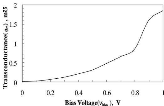
Figure-6 Variation of  $g_m$  with  $V_{bias}$  of VCCCTA
