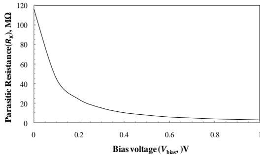
Figure-5 Variation of  $R_x$  with  $V_{bias}$  of VCCCTA
