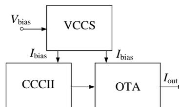
Figure-2 Block diagram of VCCCTA
