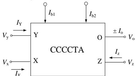
Figure-1 Block diagram of CCCCTA
