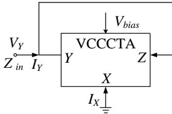
Figure-4 VCCCTA as transresistor
