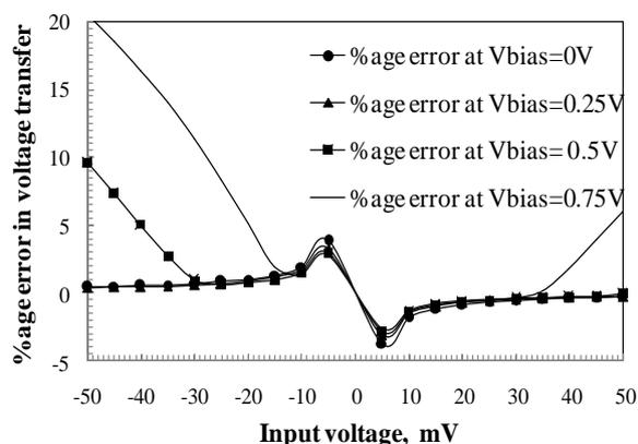
Figure-11 Percentage error in voltage transfer of VCCCTA
