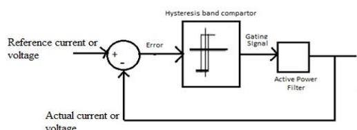
Fig 4 Block diagram of hysteresis current controller
