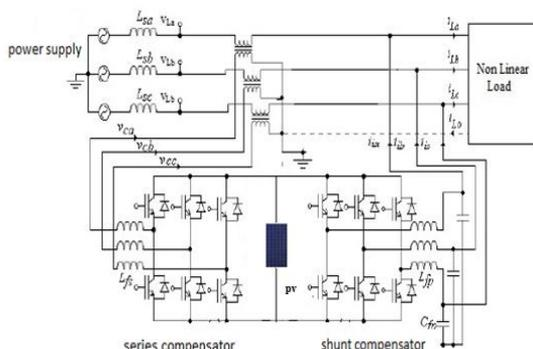
Fig. 1 Series and Shunt compensators (UPQC)
