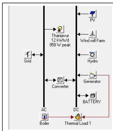
Fig.7 The simulation model of the hybrid energy system based charging station.
