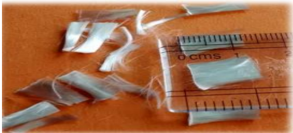
Figure:2 Polypropylene fibre showing 12 mm average size
