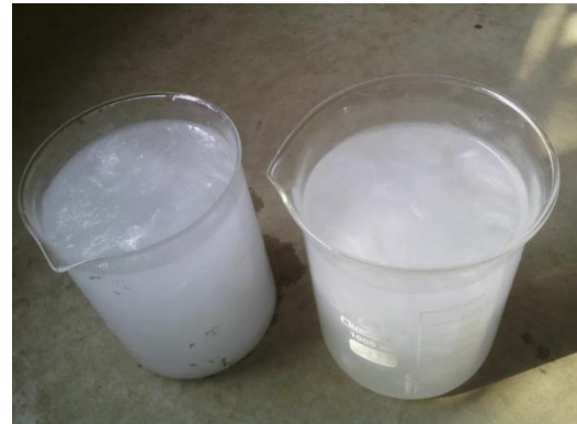
Figure:3 Dispersion of PP fibre in NaOH solution
