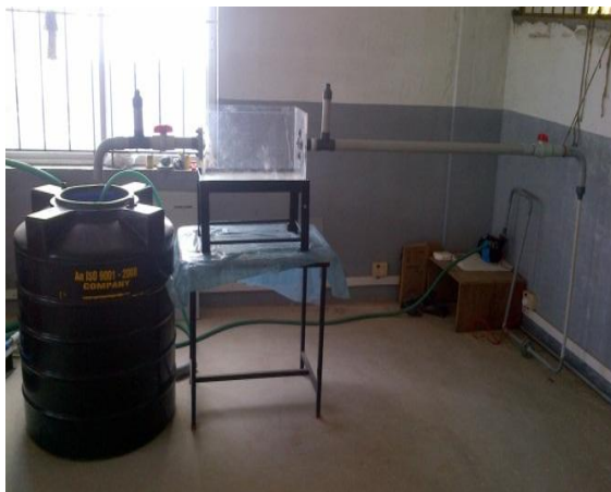
Fig-2 Experimental Setup of a Water Tunnel
