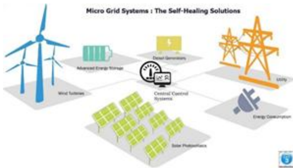
Fig. 5. Microgrid system with SCADA
