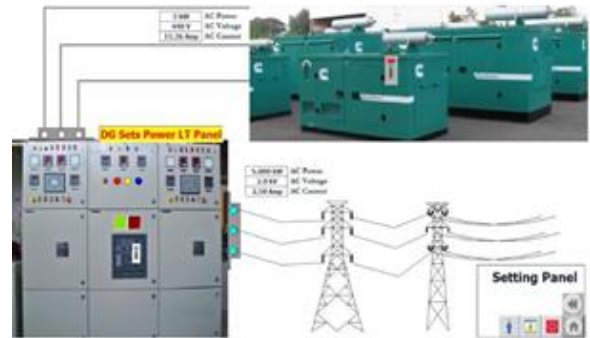
Fig. 8. Diesel system SCADA
