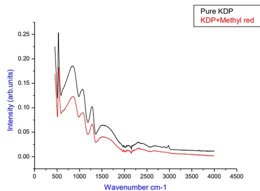
Figure 3. FTIR Spectra of (a) Pure KDP and (b) Methyl red doped KDP Crystals
