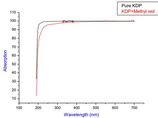
Figure 4. UV-Visible Spectra of (a) Pure KDP and (b) Methyl red doped KDP Crystals
