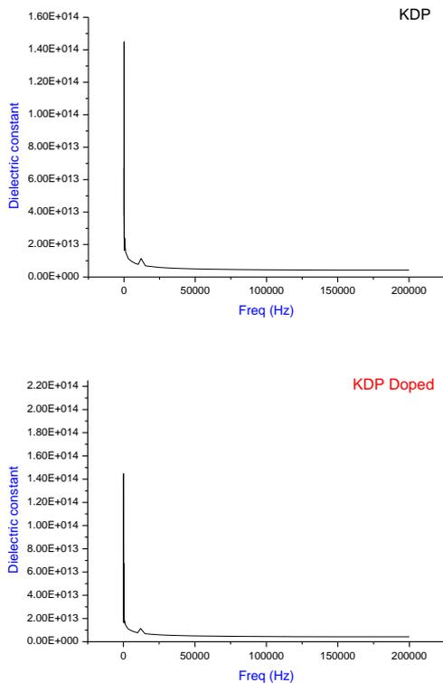
Figure 6. Dielectric constants for pure and doped KDP crystals
