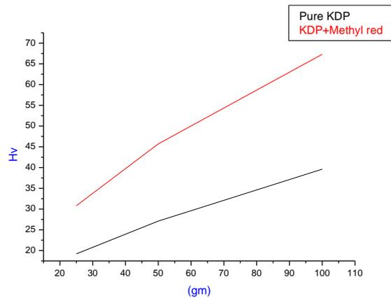
Figure.5. Variation of Hv with load for pure and Methyl red doped KDP crystal
