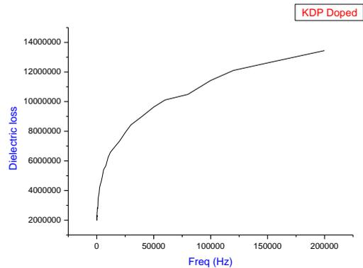
Figure 7. Dielectric losses for pure and doped KDP crystals
