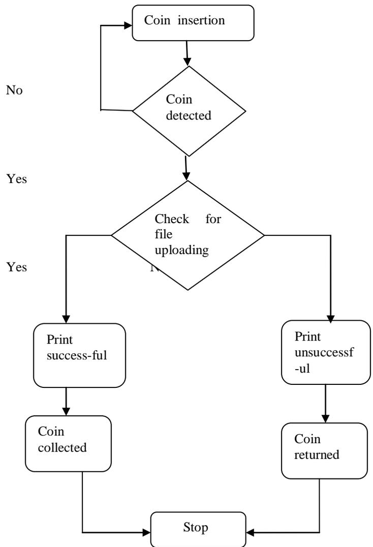
In this coin mechanism process we first insert coin. Then we check for coin is valid or not if not then user gets the instruction yo insert the coin again.
