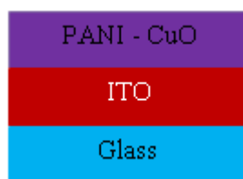
Fig7. (A) Device structure of polymer solar cell
