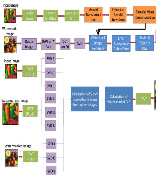
**Figure. 3.1** Proposed Copy right Water marking process
