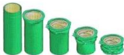
Fig.9 Deformation model of Reinforced Model of Circular Crash Tube. Ref. [7]
