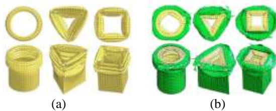
Fig.8 Deformation models of (a)Only Metallic tube (b)Reinforced Metallic Tube. Ref. [7]
