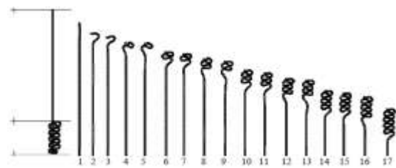
Fig 5. Deformed and Undeformed tube sides. Ref[3]
