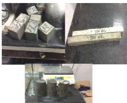
Figure 1 plain micro concrete cube, beam and cylinder specimens
