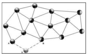
Figure 3 Wormhole created by node X'
