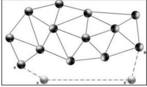
Figure 4 Longer wormhole created by two collision nodes X and X'
