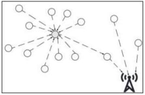
Figure 8 Sinkhole Attack
