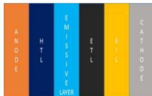
Fig.1 schematic device structure of OLED
