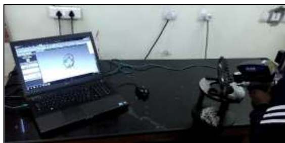
Fig. 2: Sprocket specimen scanned using FaroArm scanner
