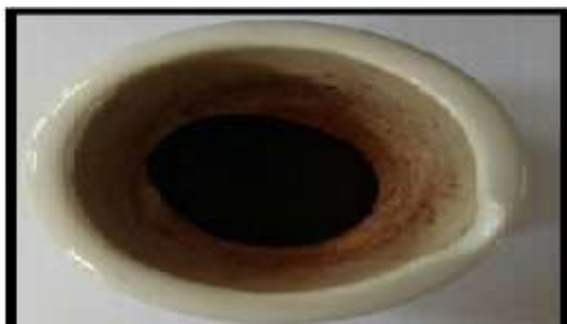
Fig 1: Synthesized Fe 3 O 4 iron oxide nanoparticles from the seaweed Gracilaria edulis
