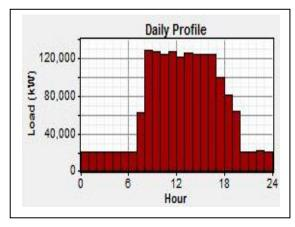
Fig. 8 The daily average thermal load profile in kW.
