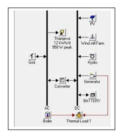
Fig.7 The simulation model of the hybrid energy system based charging station.
