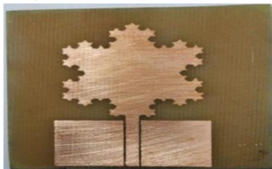
Fig.4. Fabricated Koch snowflake fractal antenna
