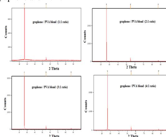
Fig. 2 XRD spectra of graphene+PVA blend in different composition
