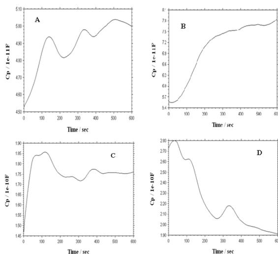
Figure 9. Plot of Capacitance Vs time for graphene - PVA thin film (1:1, 2:1, 3:1, 4:1).
