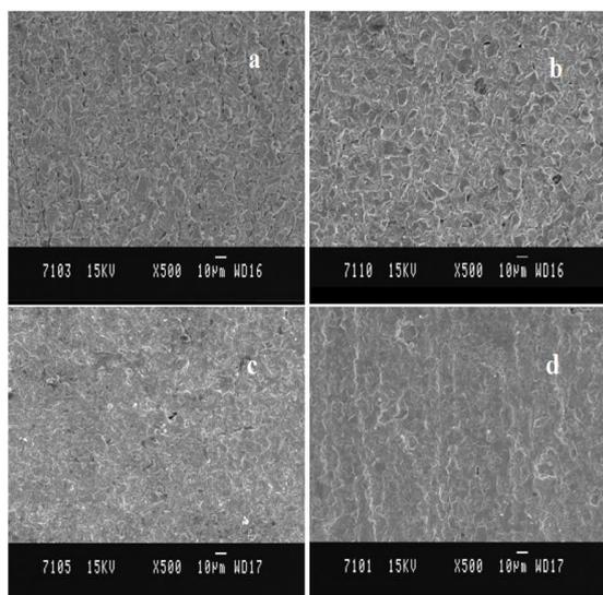
Fig.3 SEM image of graphene+PVA blend in different composition a) 1:1, b) 2:1 c) 3:1, d) 4:1
