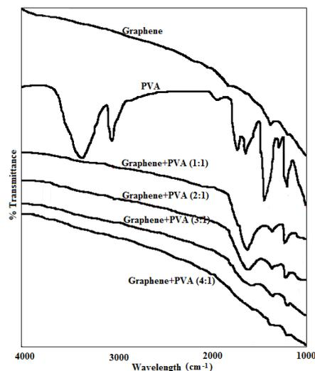
Fig. 1 FTIR spectra of graphene, PVA, graphene+PVA blend in different composition
