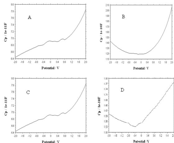
**Figure 8** Plot of Capacitance Vs Potential for graphene - PVA thin film(1:1, 2:1, 3:1, and 4:1)
