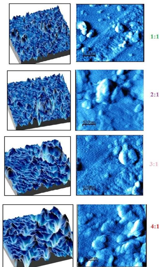
Fig. 4. AFM image of graphene - PVA thin film(1:1 ratio)
