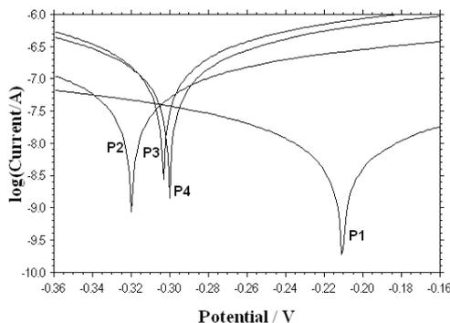
**Figure 7** Tafel plot of graphene - PVA thin film (1:1, 2:1, 3:1, 4:1)
