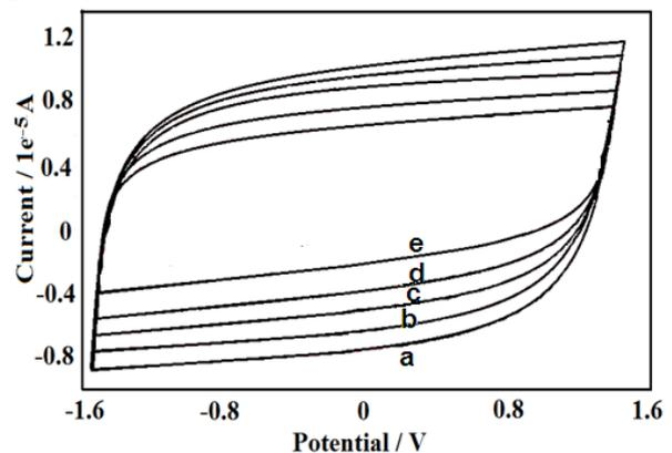
Fig. 6. Cyclic voltammetry (CV) curves of a) graphene and graphene - PVA blend thin film b) 1:1 c) 2:1 d) 3:1 e) 4:1
