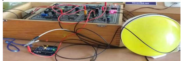
Fig: 3 Respiratory monitoring system at the time of inhalation (balloon)
