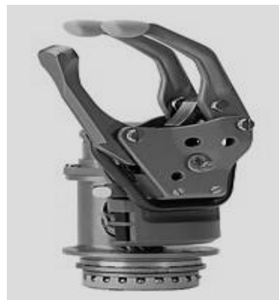
Fig. 3 Diagram of EMG Controlled Otto-Bock arm.
