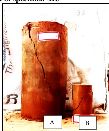
Figure 11: Failure pattern of UCS specimens for combination Soil+10%FA (A) Large-scale, (B) Small-scale
