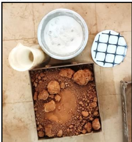
Figure 3: Materials used to prepare geogrid-reinforced flyash-modified soil
