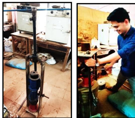
Figure 7: Arrangement of compaction and extraction of large-scale UCS specimen mould.
