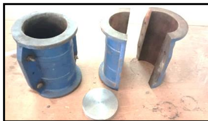
Figure 5: Mould used for Large-scale UCS specimen preparation of 100 mm in diameter and 20 mm in height
